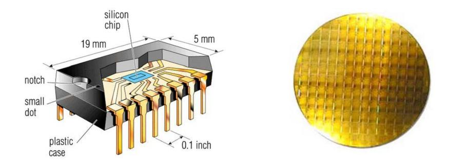
Electronic Circuits are (mostly) made by Silicon Integrated Circuit (IC) Technology → Microelectronics
